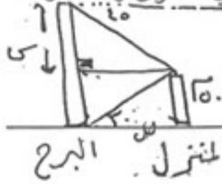
$$\left. \begin{aligned} S &= 86.6 \approx 87 \text{ م} \\ \text{ارتفاع البرج} &= 50 + 87 = 137 \text{ م} \end{aligned} \right\} \begin{aligned} \frac{50}{S} &= \tan 30^\circ \\ S &= 86.6 \approx 87 \text{ م} \end{aligned}$$
